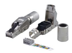
IKCOM plug is made of fully sturdy metal housing. The plug is designed to be simple and easy to be terminated with the twisted cables at field. The IDC is designed to accommodate different diameter conductors up to 22AWG. All eight conductors are terminated at same time when the wire cap is squeezed by plier. This process ensures consistent, reliable termination.
