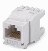
Category 6 unshielded keystone jack is designed for superior performance and easy assembly, meets and exceeds ANSI/TIA-568.2-D and ISO/IEC 11801 2nd edition Category 6 standards, supporting Gigabit Ethernet application and beyond. Narrow width design fits 24 ports in one unit panel for most efficient use of 1U panel. Jacks are available in 9 colors to match housing or allow color-coded designation port in compliance with TIA-606 requirements.
